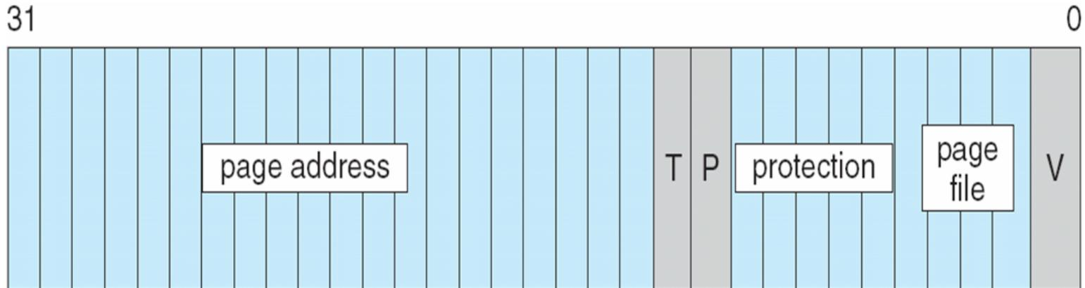
5 bits for page protection, 20 bits for page frame address, 4 bits to select a paging file, and 3 bits that describe the page state.  $V = 0$
